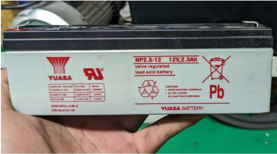
BACKUP BATTERY FIRE ALARM PANEL
