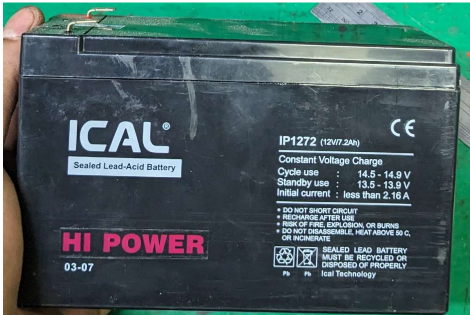
UPS BATTERY AMS Aconis
